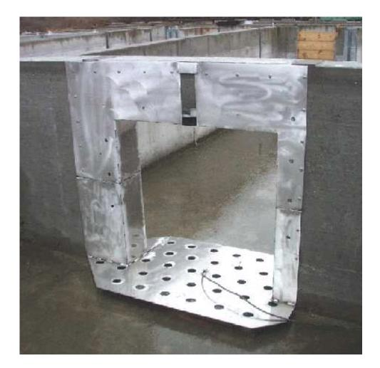
Figure 2. Photo of the alternate continuous RF shield (note welded strip at the top of the shield) that will be installed into the fish ladders during FY01. When shields are installed at the dams, the floor sections will be 8 inches beneath the fish ladder floor (not flush with the floor as shown in the photo).
