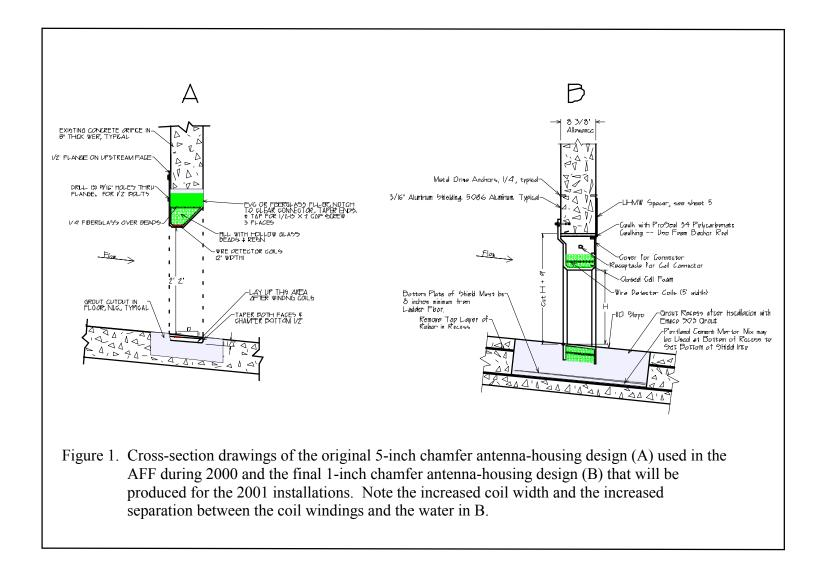
The COE and the NMFS regional office agreed in July 2000 that all antenna housings installed throughout the FCRPS could have 1-inch chamfers on both the upstream and downstream sides. However, when the first antenna housings were fabricated to incorporate 1-inch chamfers for the 26-inch orifices, the antennas performed so poorly at the Pasco test facility that we concluded they should not be installed into the AFF.
