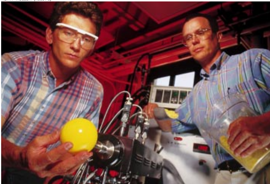
Chemical engineer J.L. Willett (right) feeds corn-flour-based stock into an extruder as entomologist Robert Behle assists with the spherical mold during experimental production of apple decoys for controlling apple maggot flies.
