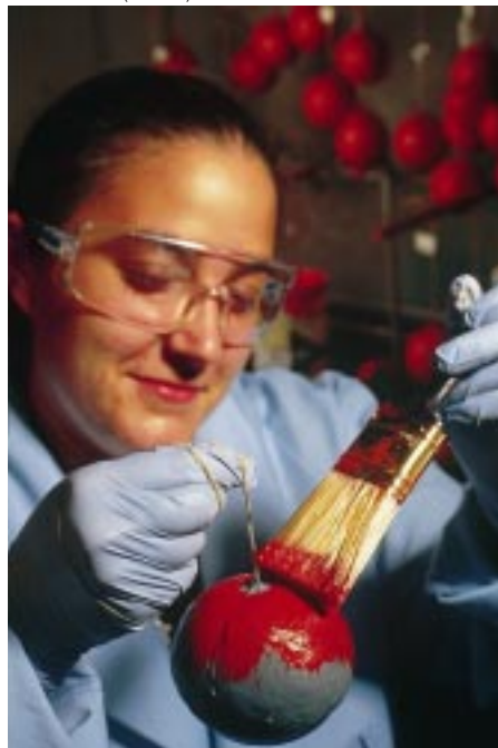
Painting the apple decoy is an essential step in the production of this insect control device. Above, technician Erica Bailey applies the final coat of paint that provides the appropriate color to attract the apple maggot fly.
