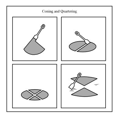
Figure C.2-2. Procedure for coning and quartering.
