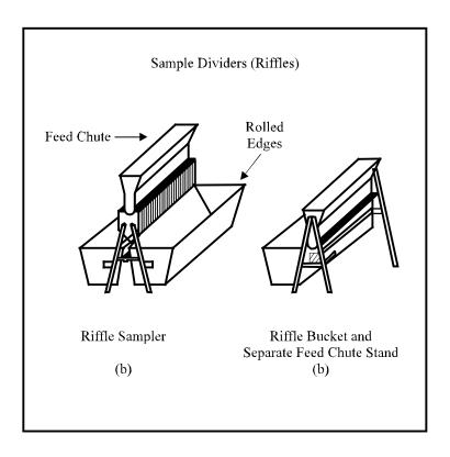
Figure C.2-1. Sample riffle dividers.
