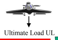
Ultimate Load is Limit Load multiplied by a Factor of Safety per 25.301(a). The minimum Factor of Safety is 1.5 per 25.305. The structure is to sustain these loads without failure per 25.305(b)
