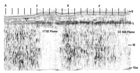
Figure 2: Ground penetrating radar profile of Line 14 showing the strong amplitude shadow caused by the proximal end of the neighboring FT-02 plume, and the somewhat weaker shadow at the right end caused by the OT-16b plume. Source: [8]
