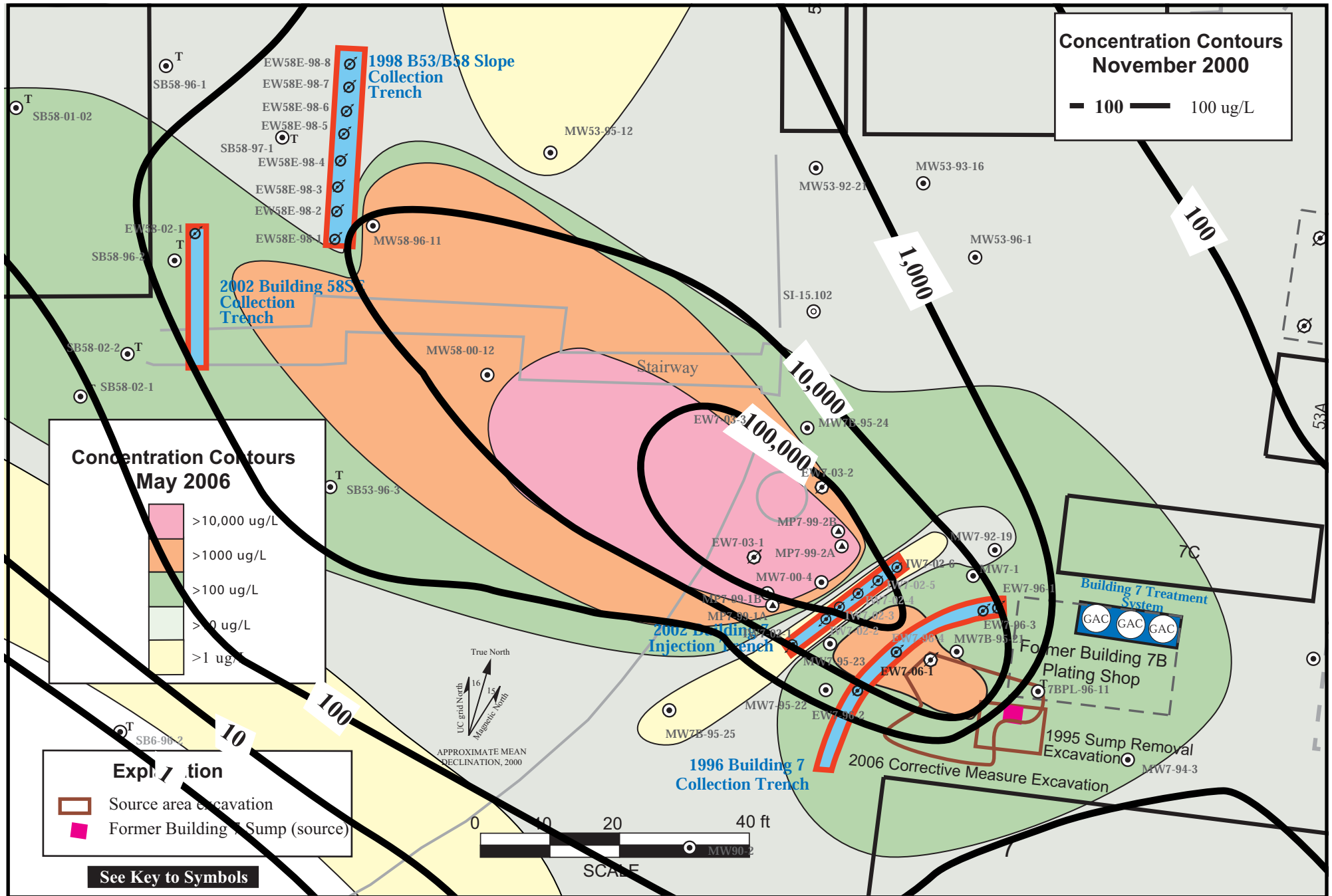
Figure 3.3-18. Total VOCs in Groundwater, Source Area Old Town Groundwater Solvent Plume Building 7 Lobe.
