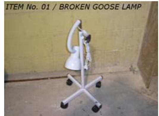
(Left): Photo of cushions for examination tables arriving at the warehouse torn due to poor packing; (right): Photo of Goose Lamp with broken stem (Warehouse in Jordan; April 2004).
