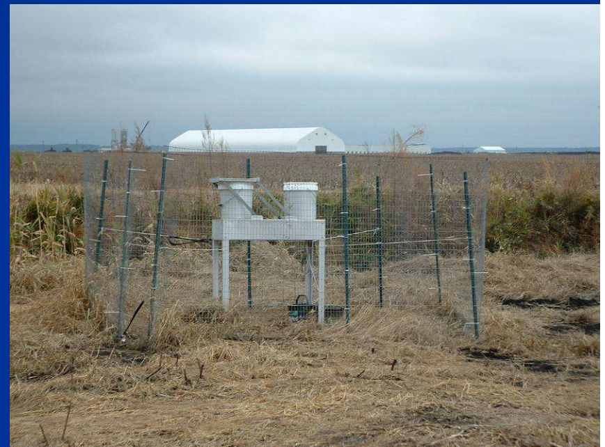
Wet deposition collection site near southern refuge boundary. Photo: S. Ward, USFWS
