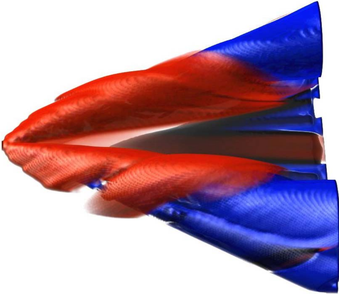
Figure 1. Visualization offers the ability to “see the unseeable.” This image shows visualization of coherent flow structures in a large scale delta wing dataset: Volume rendering of regions of high forward (red) and backward (blue) Finite Time Lyapunov Exponent. Coherent structures appear as surfaces corresponding to the major vortices developing over the wing along the leading edge [2]. Occlusion is a limitation that can be addressed with cropping or clipping. (Image courtesy of X. Tricoche, University of Utah and C. Garth, University of California – Davis)
