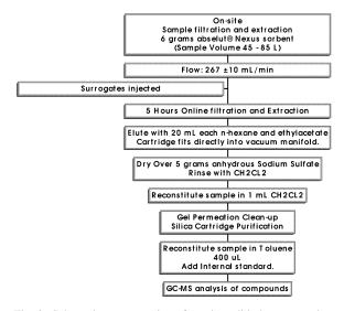
Fig. 2. Schematic representation of on-site solid-phase extraction procedure with Abselut NEXUS sorbent.
