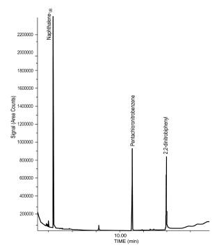
Fig. 3. Total ion chromatogram of field blank.
