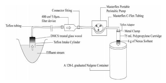
Fig. 1. On-site solid-phase extraction assembly.
