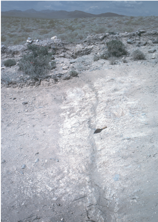
Figure 40. Surface rupture from a late Holocene coseismic event exposed in vesicular A soil horizon that underlies modern desert pavement on scarp just south of trench CF2 across the Windy Wash Fault in the Yucca Mountain area, southwestern Nevada (figs. 1, 2). Fissure is 8 to 15 cm wide; hand trowel is 21 cm long.
