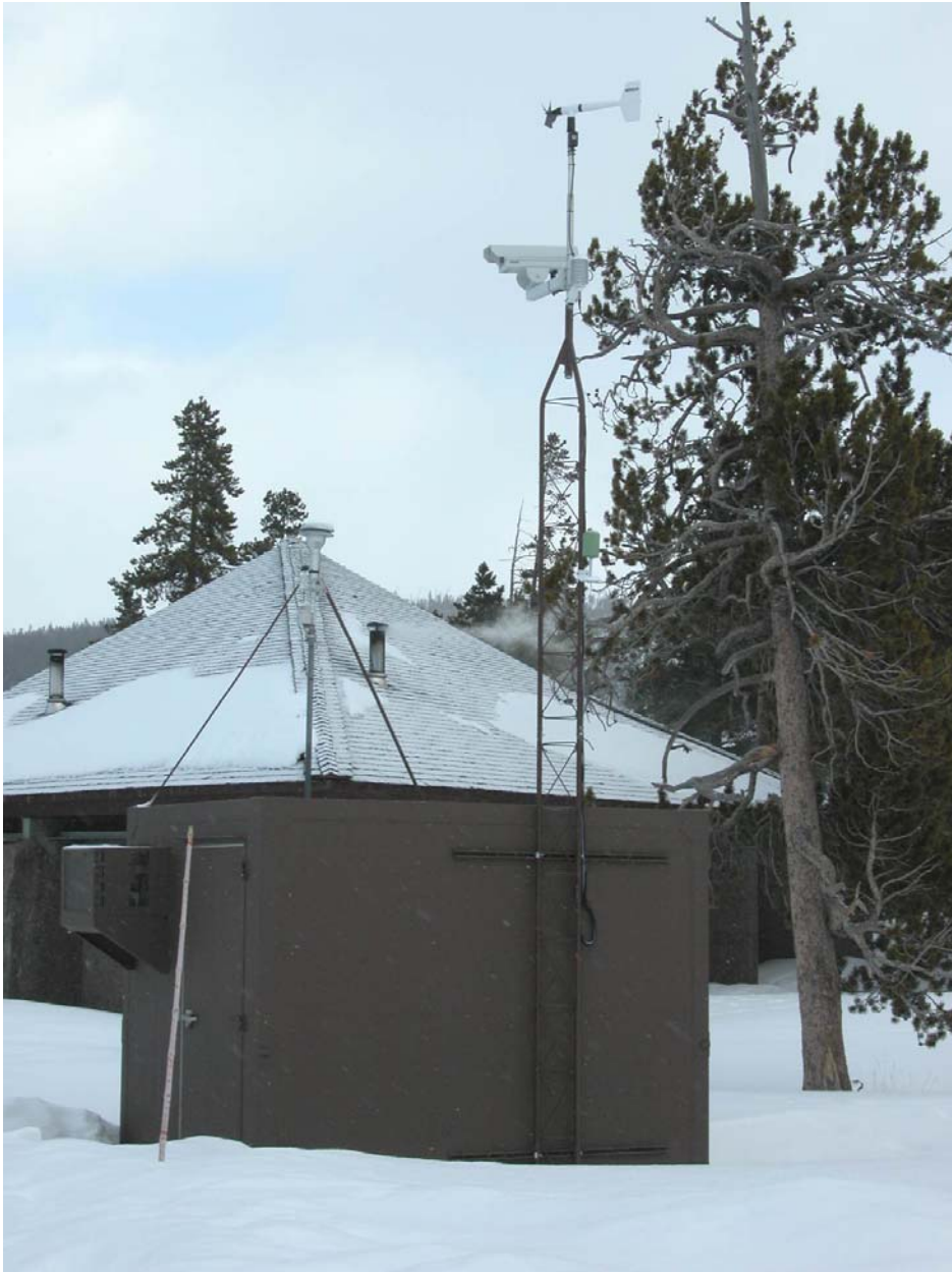
Picture of the monitoring shelter at Old Faithful with the warming hut in the background. Smoke is seen blowing away from the monitoring station in the SW winds. The digital camera housing can be seen on the tower.
