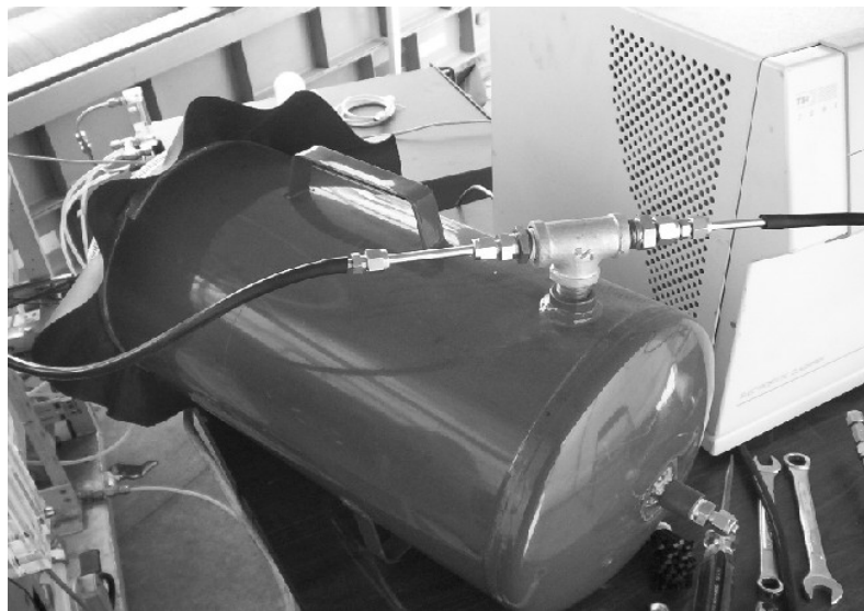
Figure 12: Exhaust Pulsation Damper
