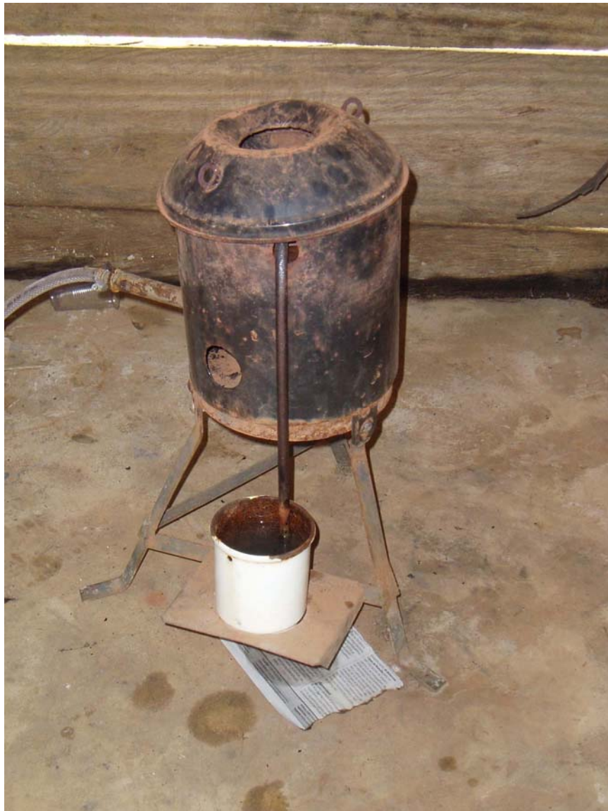
Figure 3. Sealable mercury retort at Mina Cabecera Santa Ynes, Huelapethue, Madre de Dios, Peru. Tube on side helps to capture some of the volatilized mercury fumes. (Photograph by William E. Brooks)
