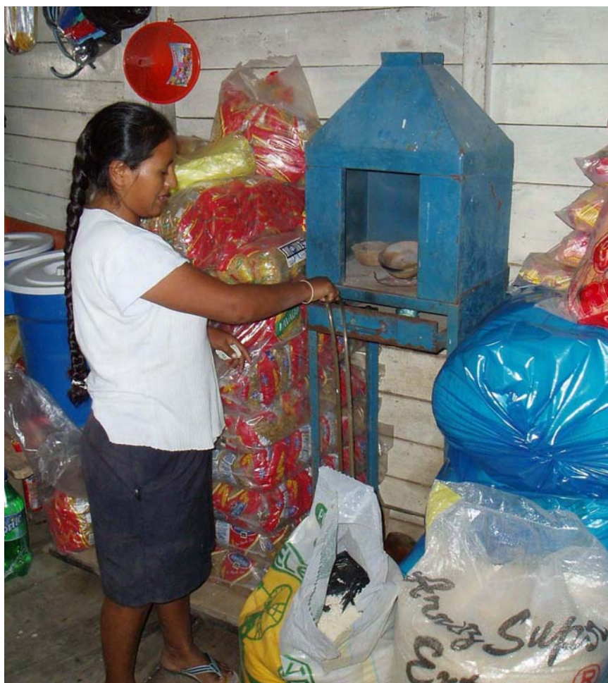
Figure 2. Unvented mercury retort for gold processing in a grocery store in Inambari, Madre de Dios, Peru (Photograph by William E. Brooks)
