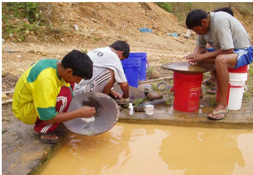
Figure 6A) Sluice and b) silvery, mercury-gold amalgam in gold pan (batea) in foreground at Mina Cabecera Santa Ynes, Huelphue, Madre de Dios, Peru. (Photographs by William E. Brooks)
