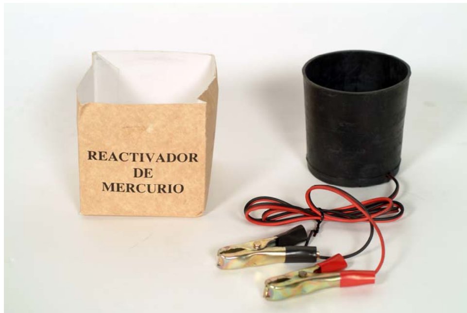
Figure 5. Mercury reactivator for cleaning and recycling mercury by using electricity from a 12 volt battery. (Photograph by William E. Brooks)
