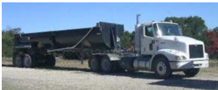
Figure A - Semi-Trailer End Dump Truck (Note: prohibited from dumping cohesive materials)
