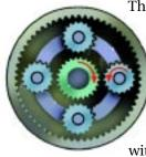
The THS transmission is not a conventional automatic transmission. There is only one gear set, with no clutch,
