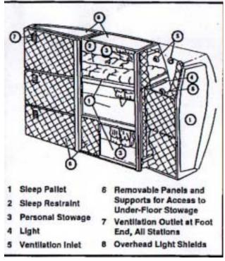
The Shuttle orbiter can be outfitted with up to four bunks, three horizontal and one vertical.
