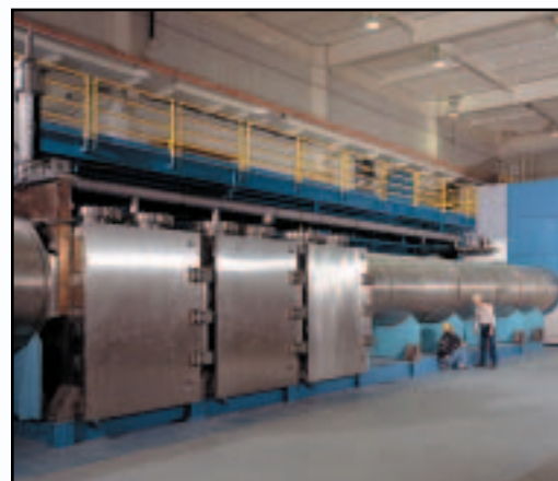
Livermore's plant-scale uranium separator system was one of the largest technology transfer projects in the Laboratory's 50-year history.
