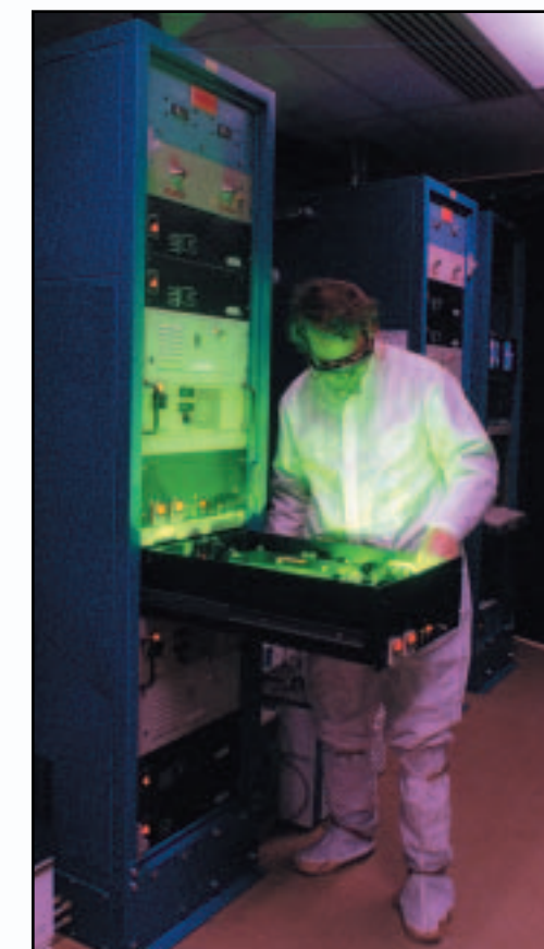
A technician works with the diode-pumped solid-state green laser developed for U-AVLIS. The technology is being used for precision machining and many other applications, such as pumping ultrashort-pulse lasers, creating laser displays, and treating disfiguring skin conditions.
