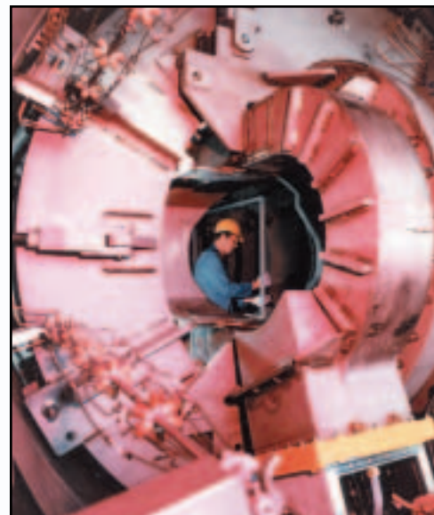
Great success in the Tandem Mirror Experiment (above) led to TMX-Upgrade (far left and left). The vacuum vessel was enlarged, and new end coils were installed in an attempt to demonstrate the thermal barrier concept and improve performance over TMX.
