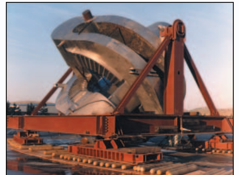
One of the yin-yang magnets for MFTF-B being moved into Building 431. The magnet system for MFTF-B was the largest superconducting system ever built.
