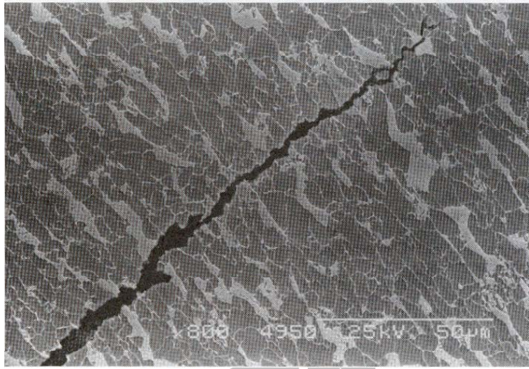
Figure 4-4 Transgranular Cracking in Pipeline Steel (Revie 2000)
