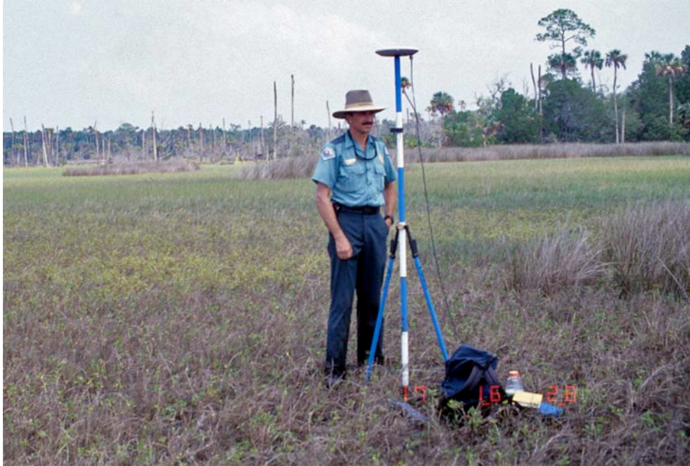
Photo 4 Differential GPS roving antenna in high marsh at Lukens Creek.
