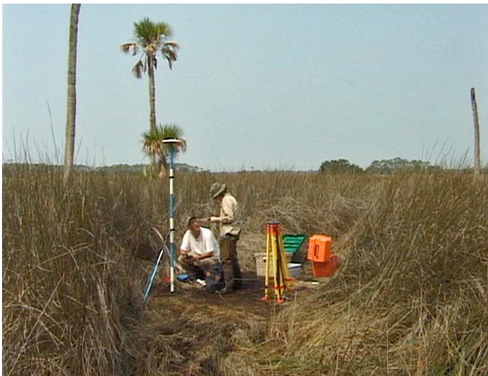
Photo 5. Roving antenna and geodimeter in black-needlerush marsh.
