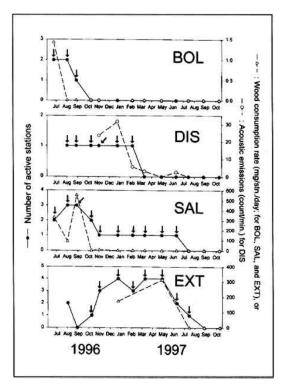
Fig. 4. Termite activity for the four populations, BOL, DIS, SAL, and EXT, found on the two ground floors at the pedestal of the Statue of Liberty National Monument. Activity is expressed by wood consumption rates (open triangles with dotted line), acoustic emission counts (open circles with dotted line), and number of monitoring and baiting stations with live termites (black circles with solid line). Arrows depict applications of baits containing 0.5% hexaflumuron.
