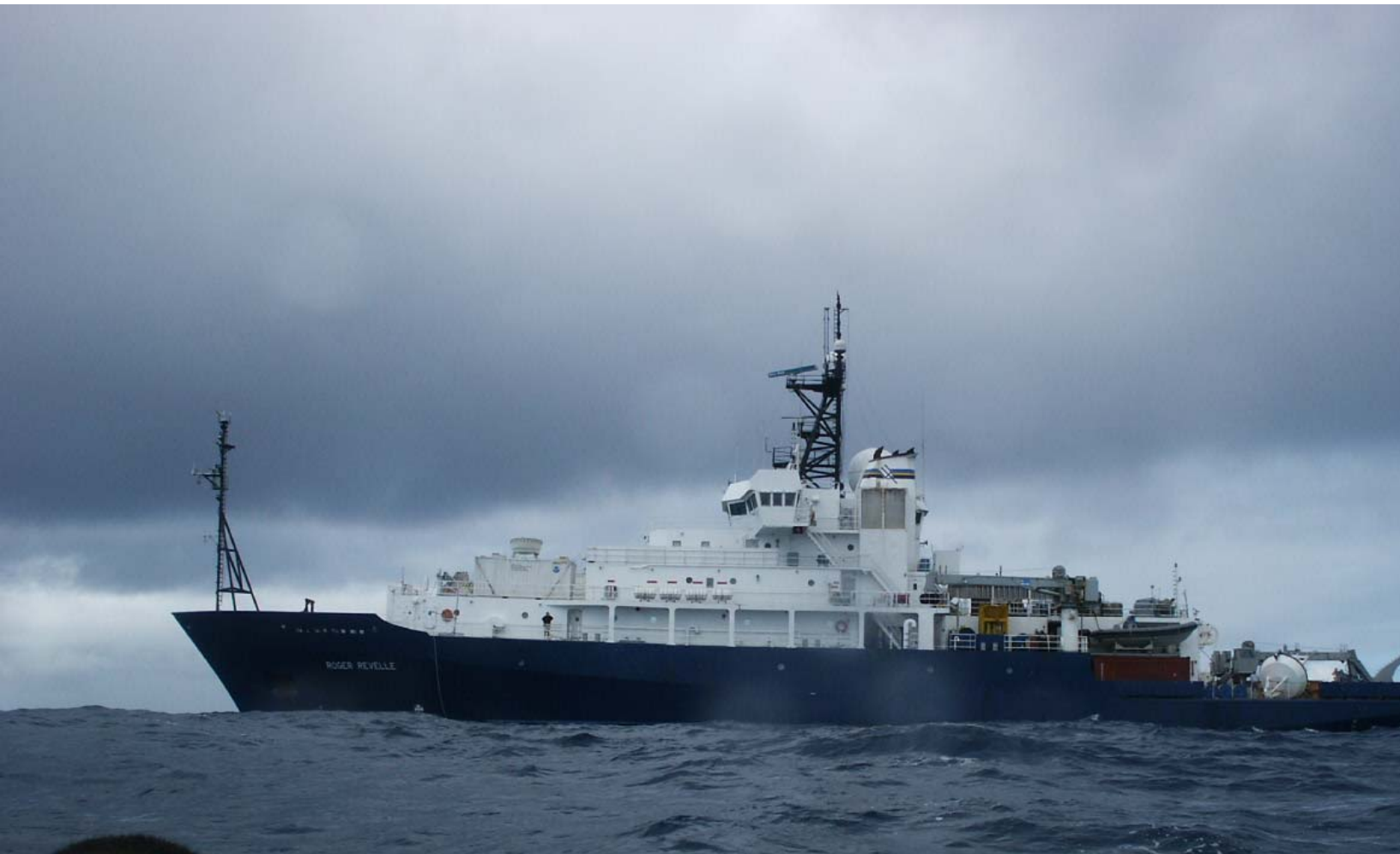
Figure 1. The Scripps Oceanographic Institution Research Vessel Roger Revelle at 20 S Latitude 85 W Longitude supporting NOAA's Ocean Observations and Climate Variability programs. ETL's seagoing flux system is on the mast on the bow; the cloud radar and microwave radiometer container is forward on the second white level (you can see the antenna on top). The replacement WHOI climate buoy is the round white object sitting low on the stern. The buoy is lying on its side are you are looking at the bottom.
