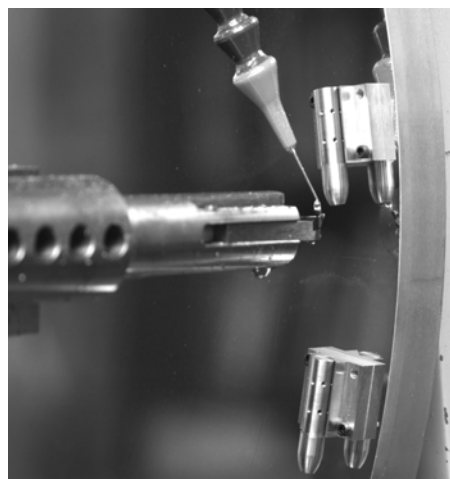
Figure 4: Machining lands using diamond turning machine.
