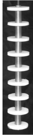
Figure 2: OFHC copper blanks, separated by spacers, destined to be electroplated and then machined into reference bullets.
