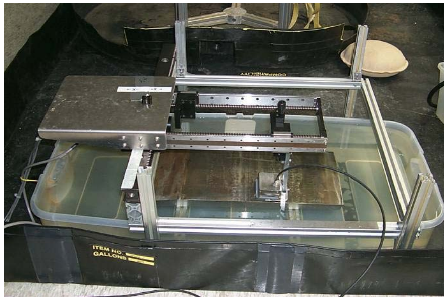
Figure 6.1 Laboratory Setup for Phased Array Data Acquisition on Westinghouse Owners Group Specimens
