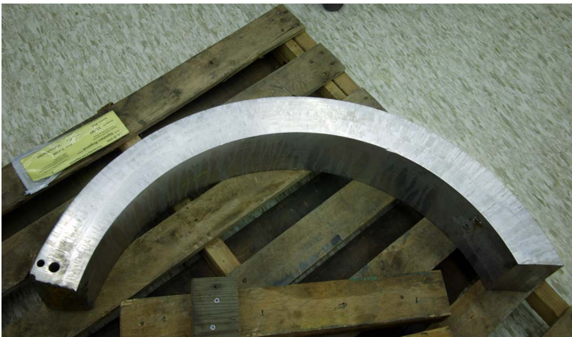
Figure 4.1 Centrifugally Cast Stainless Steel Piping Segment Loaned by IHI Southwest Technologies, Inc.
