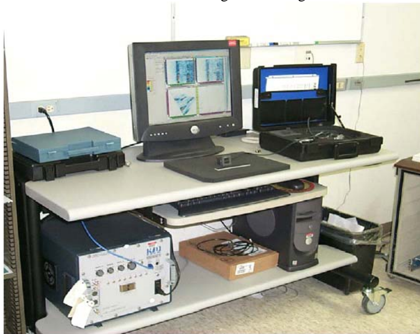
Figure 2.5 Typical Phased Array System Components
