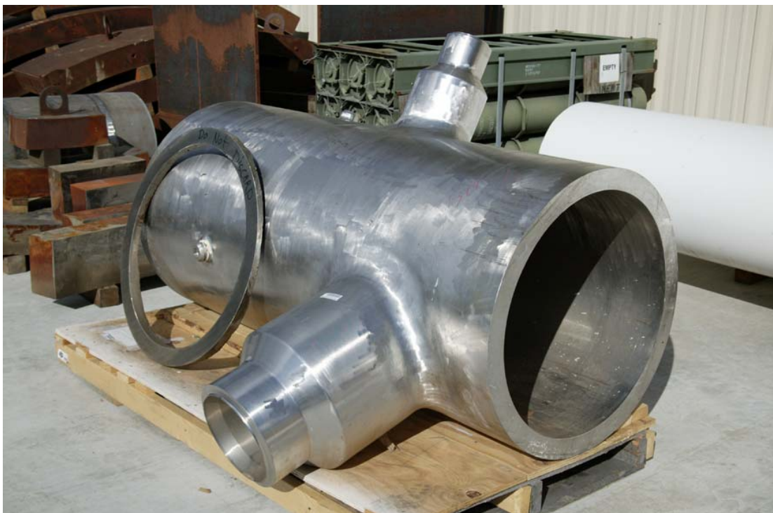
Figure 4.5 Large Blank Spool Piece on Late-Vintage CCSS Piping from Cancelled Spanish Plant on Loan to PNNL by EPRI
