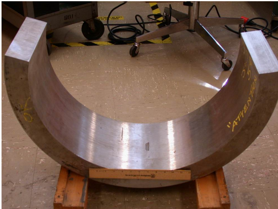
Figure 4.4 Westinghouse, Inc. CCSS Piping Segment on Loan to PNNL
