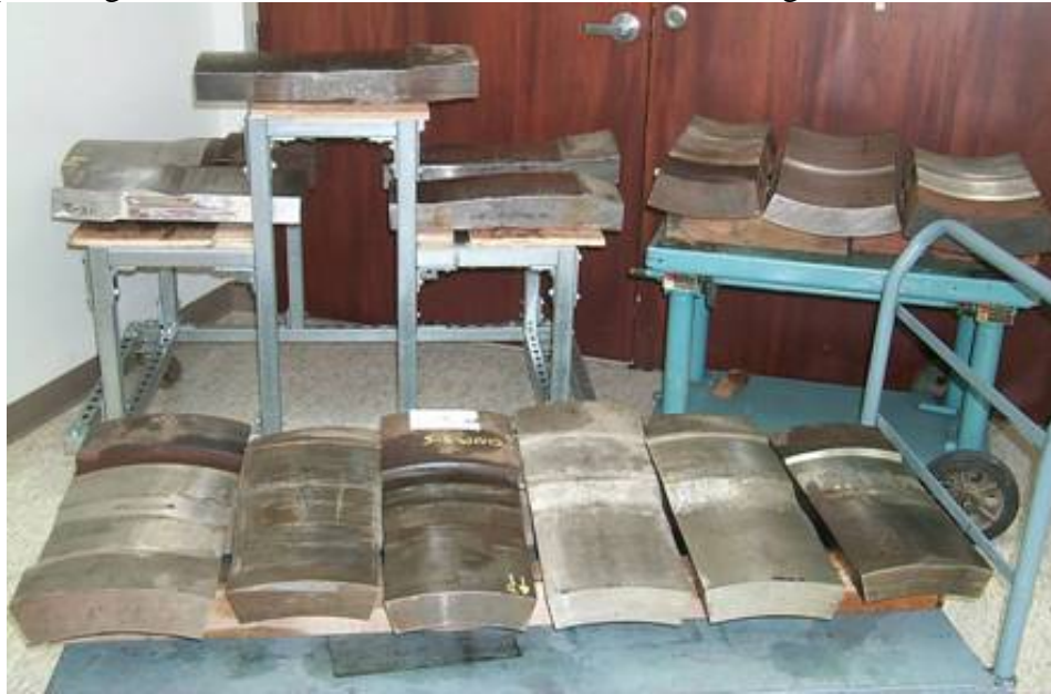
Figure 4.7 Westinghouse Owners Group Specimens Showing Varied Inside and Outside Surface Geometries Typical of Field-Installed Components
