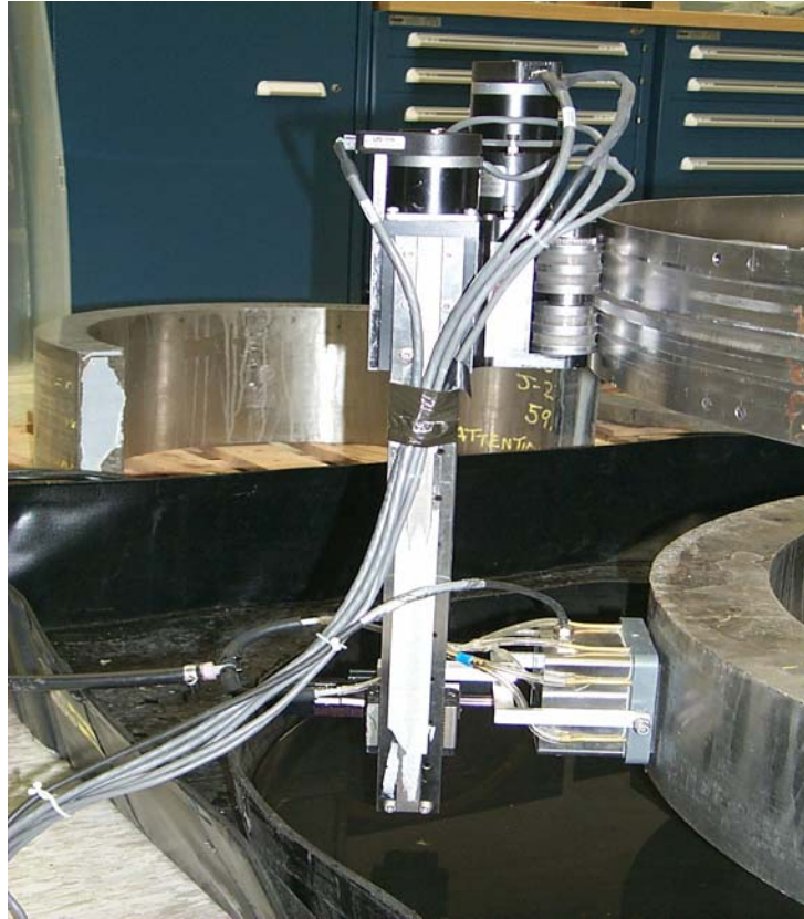
Figure 5.1 Laboratory Setup for Phased Array Data Acquisition on the IHI-SW Vintage Piping Segment
