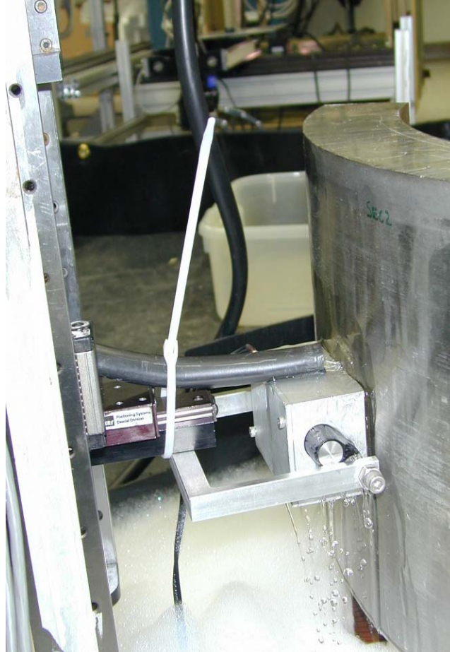
Figure 3.8 Variable-Angle Low-Frequency/SAFT Probe Shown on Westinghouse Piping Segment
