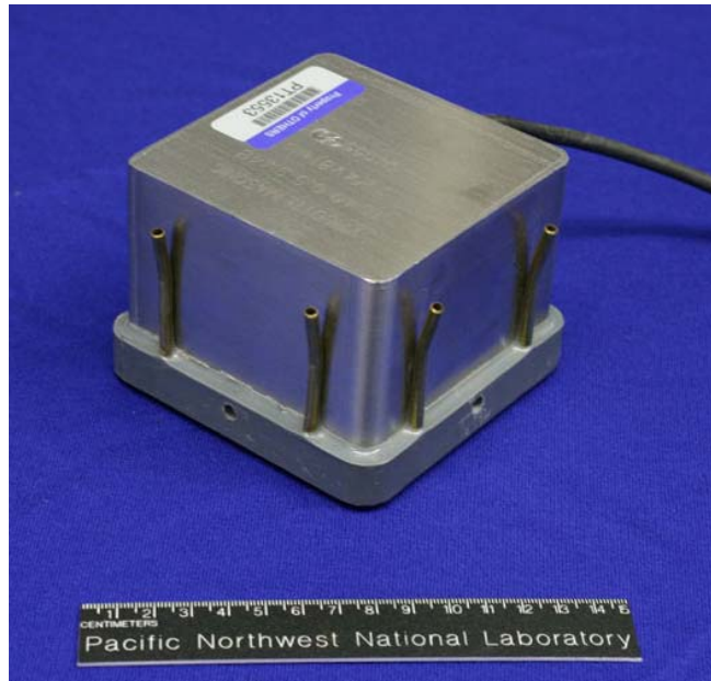
Figure 3.2 Improved Design 500-kHz Phased Array Probe
