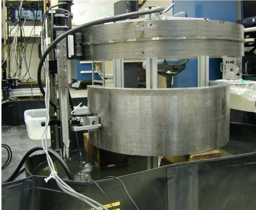
Figure 5.11 Low-Frequency Scan Apparatus for Westinghouse and IHI-Southwest Segments
