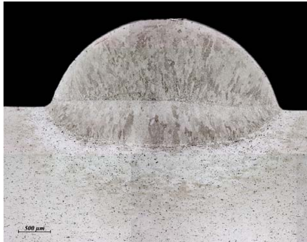
Figure 2. Microstructure of preheat pass plus single layer deposit, representative of 30 to 50 kV deposits (50 kV accelerating voltage shown).
