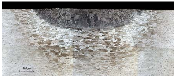
Figure 1. Representative microstructure for preheat pass only (30 kV accelerating voltage shown).
