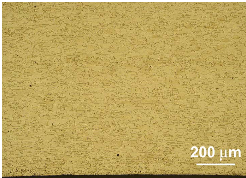
Fig. 14: Recrystallized grain structure near rolling surface of spray-rolled 2124. Sample was solution heat treated (493°C, 2 h.), cold rolled 75%, and annealed (493°C, 10 min.). Longitudinal section.
