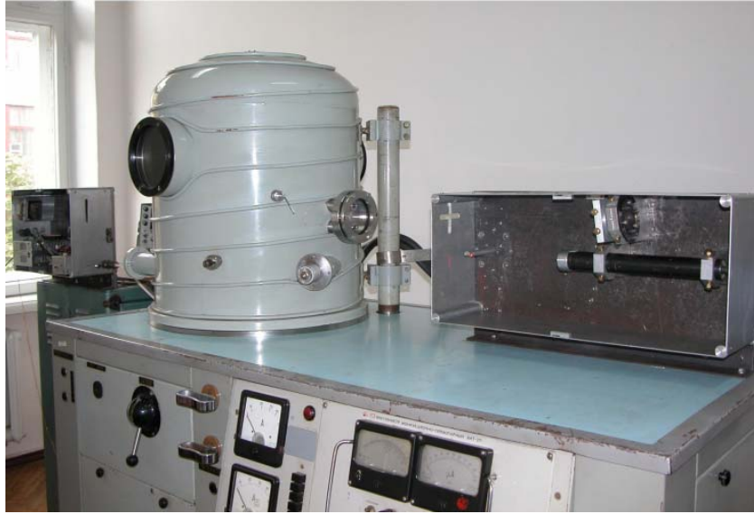
Figure 4. Appearance of the machine to study linear thermal expansion of metals
