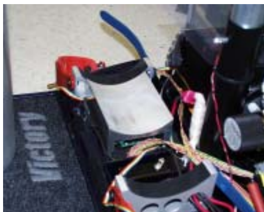
Figure 9. Machined DC-DC Converter mount / heat transfer cradle - Top view.
