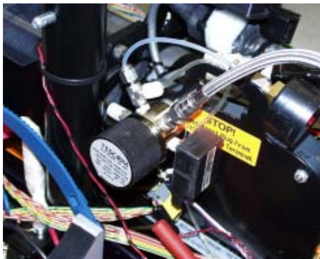
Figure 10. Piston-sensed pressure-reducing regulator.
