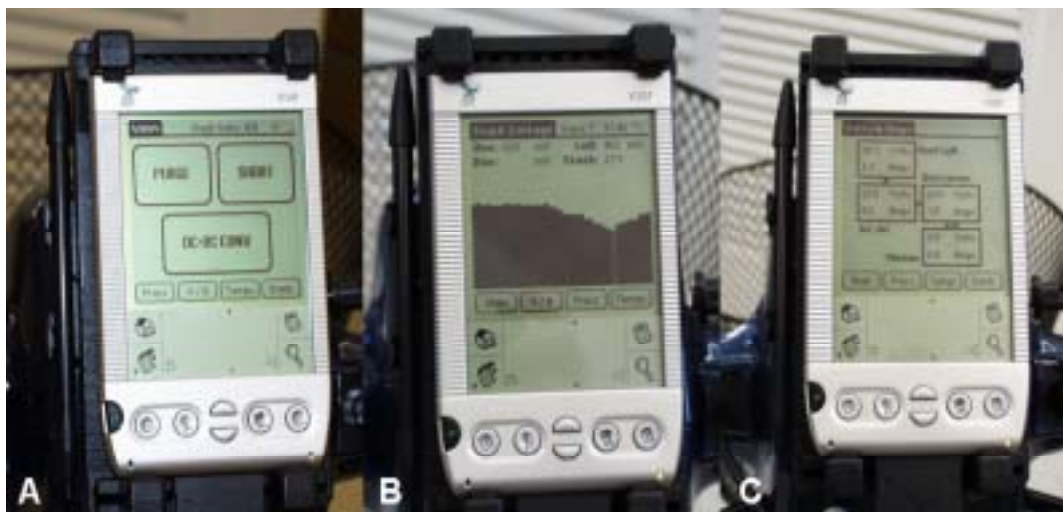
Figure 4. Scooter operator display screens. A is the main control screen, B is the stack cell voltage display showing a loaded stack, and C is the volts and amps display.
