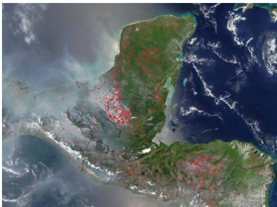
Fig. III. An example of the SERVIR fire product with fires (red dots) overlaid onto MODIS imagery.
