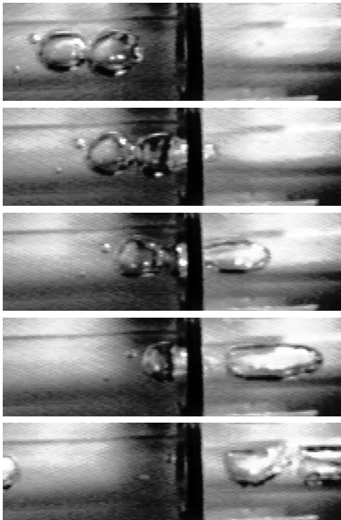
Figure 1.—Time Sequence as two bubbles flow through a 25.4 to 19 mm contraction.
