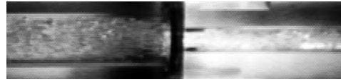
Figure 2.—Bubble flow through a 25.4 to 12.7 mm contraction. The dark band on contraction is where the gas is recirculating.
