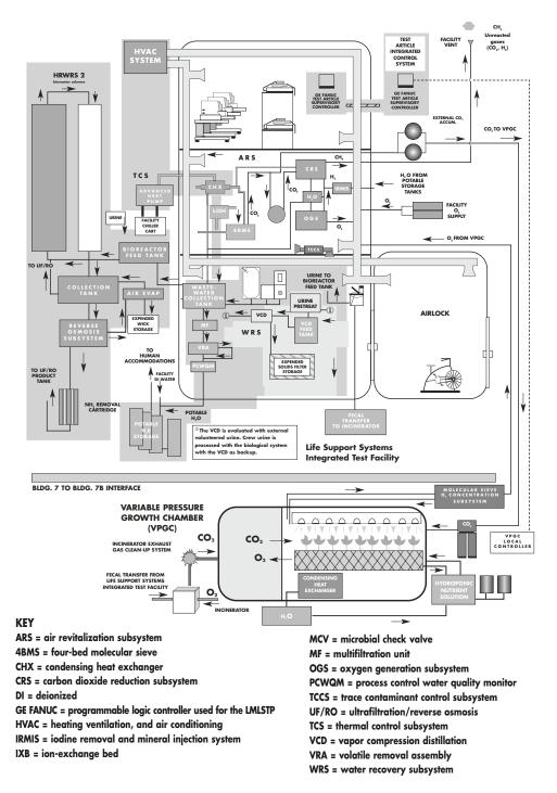
Figure 2.1-6 The Phase III, 91-day test functional schematic
