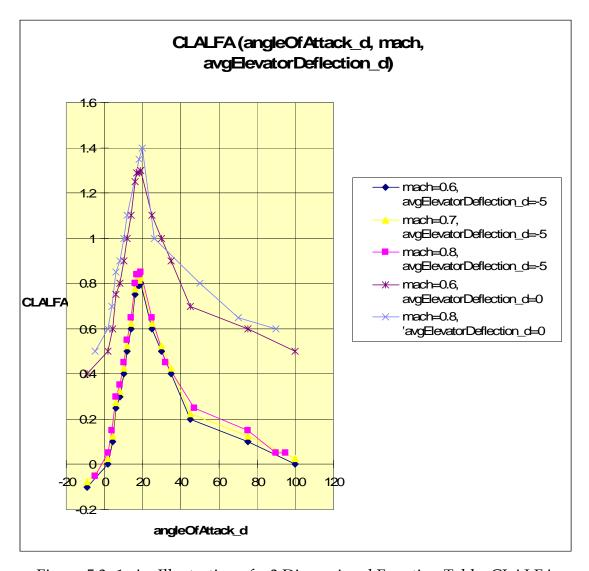
Figure 5.3 -1 An Illustration of a 3 Dimensional Function Table, CLALFA (angleOfAttack\_d, mach, avgElevatorDeflection\_d)
