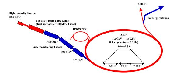
Figure 7: AGS proton driver layout.
