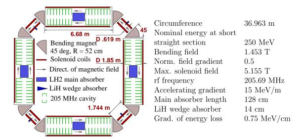
Figure 17: Layout and parameters of the solenoid based Tetra ring cooler
