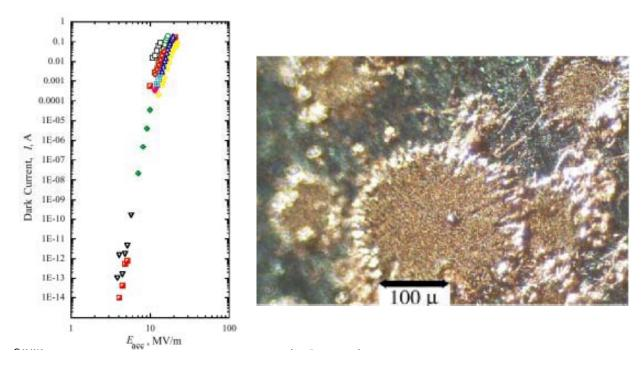
Figure 14: Dark current measurements in rf cavity in a magnetic field. Damage to the cavity can be seen.
