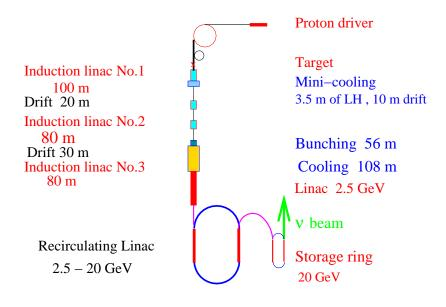
Figure 1: Schematic of the Neutrino Factory Study-II version.
