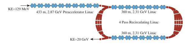
Figure 16: Accelerating system layout.
