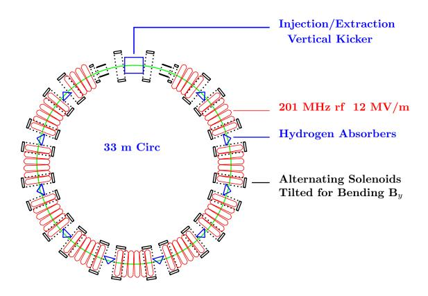
Figure 19: Layout of an RFOFO cooling ring.
