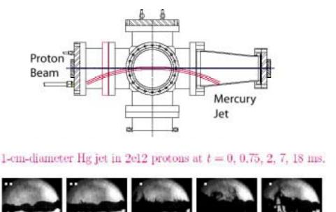
Figure 10: Targetry setup and photographs of beam hitting mercury jets at t=0,0.75,2,7 and 18 ms.
