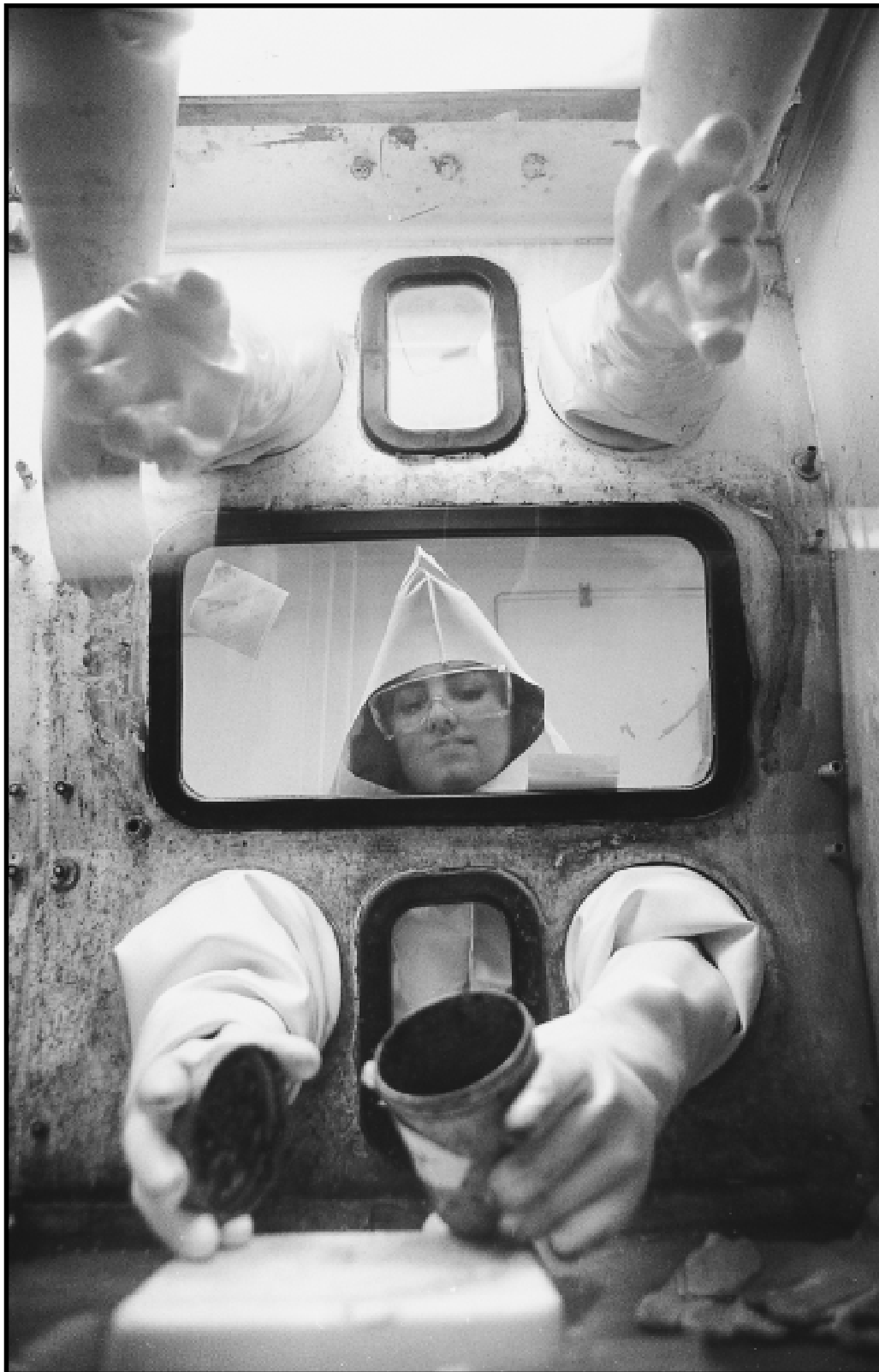
Glovebox for handling plutonium is a sealed environment kept under negative pressure and, when necessary, filled with inert gas to keep the plutonium inside from igniting in air. Safety procedures require workers to wear anti-contamination clothing and to handle plutonium through rubber gloves attached to the wall of the box. Plutonium Finishing Plant, Hanford Site, Washington. December 17, 1993.
