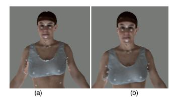
Figure 6. Results of hole filling using Tight Cocone method from front view. (a) Before filling. (b) After filling.
