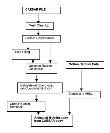
Figure 3. The structure and data flow of the process.
