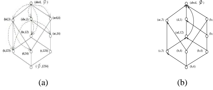
Fig. 2. (a) Irregular concepts regarding (abcd, \emptyset) , (bd, 3) and (abc, 1) . The concepts pointed by an arrow and connected to (abcd, \emptyset) ( (bd, 3)/(abc, 1) ) by dashed lines are its irregular concepts. Note that the lattice is in the full representation. (b) The same lattice in a compact representation computed by our algorithm. For each concept, a directed edge points to its base.
