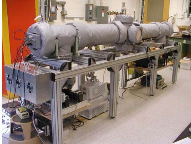
Figure 1: The Paul Trap Simulator Experiment (PTSX) is a compact laboratory experiment that studies the transverse dynamics of high-intensity beam propagation.
