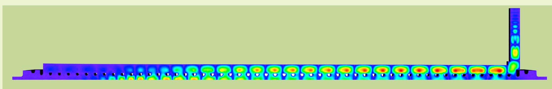
Eigenmode with high kick factor/low Q from Omega3P in 1st band of the H60VG4.
