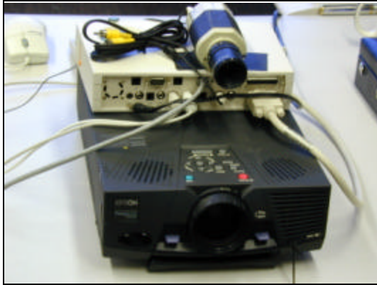
Figure 8. A Smart Projector prototype. The attached NetwinderDM 275 computer drives the Epson 7500c projector. The NetwinderDM reads frames from the camera to do a variety of measurements on the projector.
