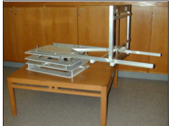
Figure 4. Intel-Princeton projector positioner with aperture modulation frame. The magnetically attached vignetting blades are easily adjusted.
