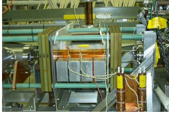
Figure 21: FRX-L with top half of \theta -coils removed, showing Kapton-wrapped quartz tube, diagnostic flux loops (white twisted cable), flux-excluder plates, and (greenish) pancake cusp coils.
