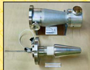
This fast-pulsing neutron source features shielded high-voltage components. Its small size and user-friendly operating characteristics appeal to university and laboratory researchers. The output is up to 10^8 neutrons per second from the deuterium-deuterium reaction.
