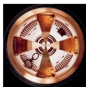
The compact and efficient radiofrequency quadrupole linear accelerator, or RFQ, is one of the keys to the ADNS project. Designing and building RFQs is a special strength of AFRD and Engineering.
