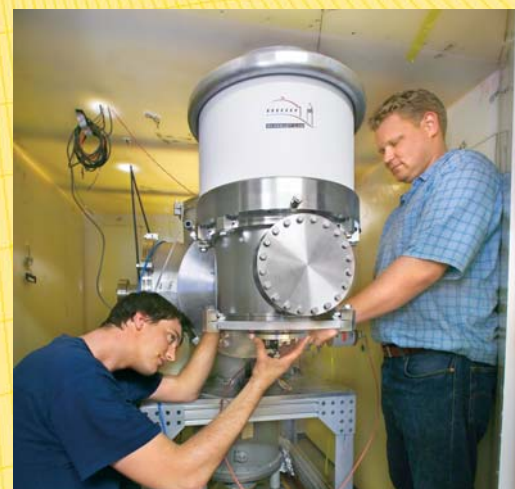
The High Output Coaxial Target Neutron Generator won a 2006 R&D 100 award. It is a high yield, continuous-beam deuterium-deuterium neutron generator that gives 1000x higher neutron yield than direct competitors. Several applications in homeland security, industry, research, and the medical field are in use or under development. This 10^{11} n/s version was delivered to the hospital/university consortium EUROSIA in Turin.
