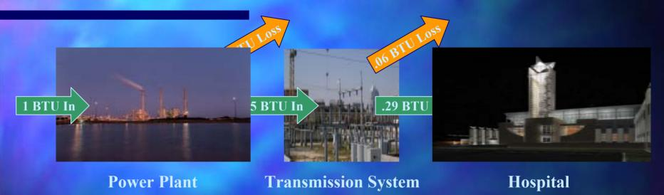
At Austin Energy's Fayette Power Station, for example, 35% of the primary fuel is converted into electricity; the remainder is lost "up the stack". An additional 6% efficiency drop occurs in transmission to the site. Overall, at the Hospital's meter, the result is roughly a 29% efficient primary fuel conversion to useful energy.
