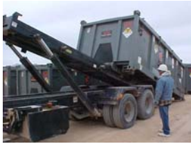
Roll-off trucks shift unstable loads to rear. (Note: the trapezoidal “dog box”)
