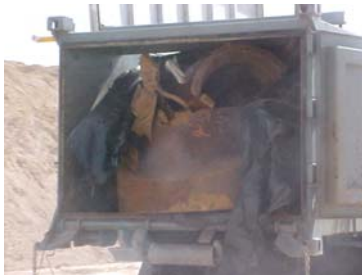
Too high in container, interfering with top of header
