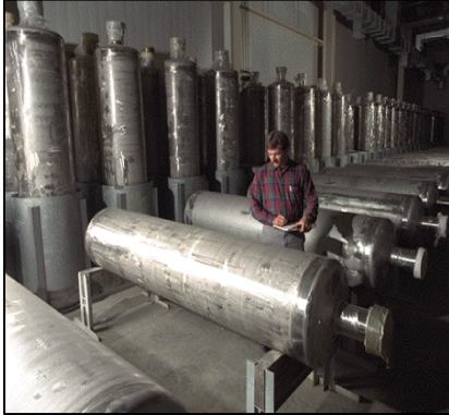
Canisters being received (prior to being filled with radioactive glass)
