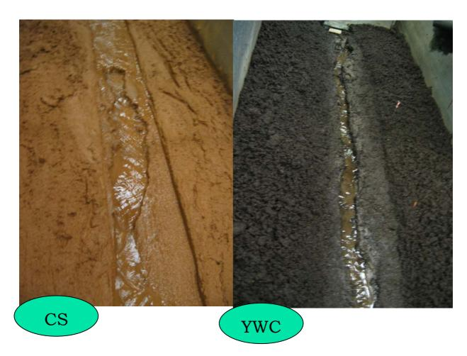
Figure 2: Rill process of on Yard waste compost and Cecil soil
