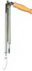
A sling psychrometer is relatively inexpensive but is not as accurate as a motor-driven model
