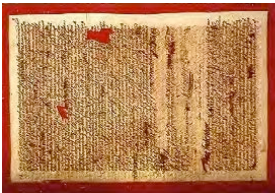
Iron gall ink can be so acidic that it "burns" through a paper sheet.
