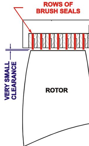
This cartoon shows the use of brush seals to provide a compliant casing for short-duration rub events ... describe brushes (brush seals typical of those used for control of secondary flowpath leakage)
