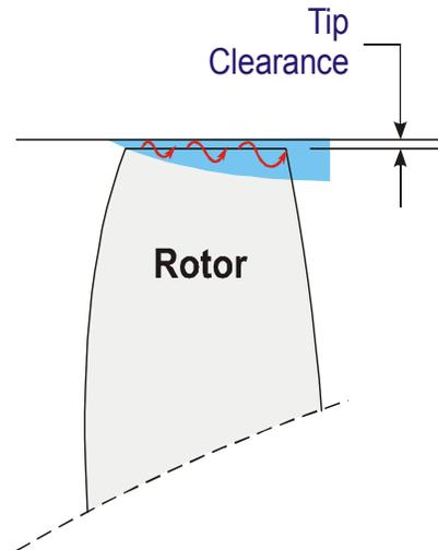
In aircraft engines, some clearance exists between rotor & casing
