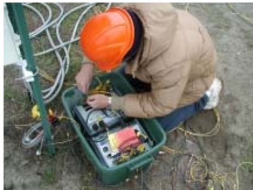
Photo 2 – receiver scanners with custom cabling
