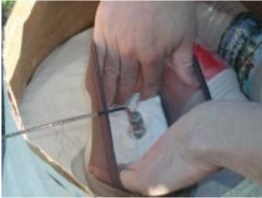
Photo 3 – Steel electrode in diatomaceous earth
