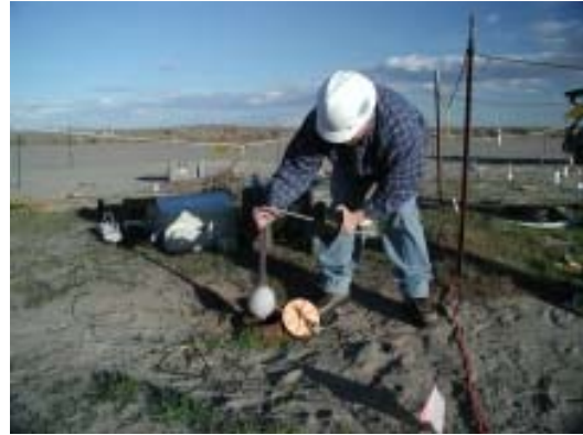
Photo 4 – Lowering electrode down casing
