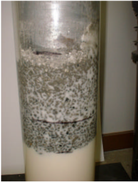
Figure 11. Photo showing the emulsion permeating the interstitial spaces of drill cuttings when loaded at 10 psi.
